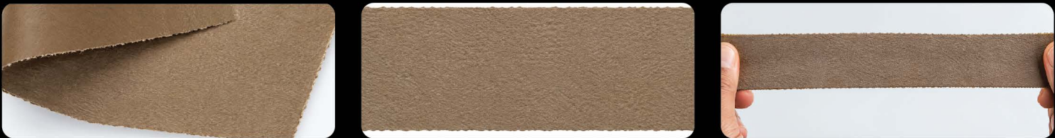
The cured film, free of its substrate — folded, flat and stretched by hand. A three-dimensional cellulose fibre network runs through it, which is why it takes that movement without tearing.
