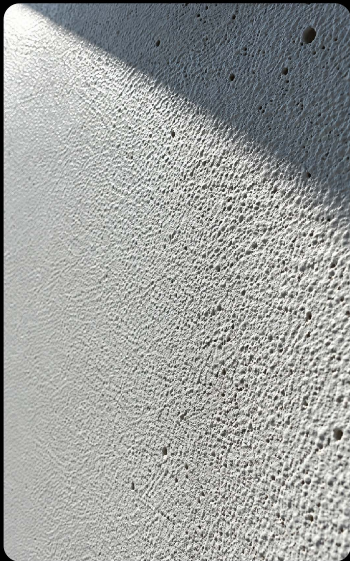
The cured film — matt, faintly textured, and the same grey whether it is going under a tile bed or lining a reservoir.
