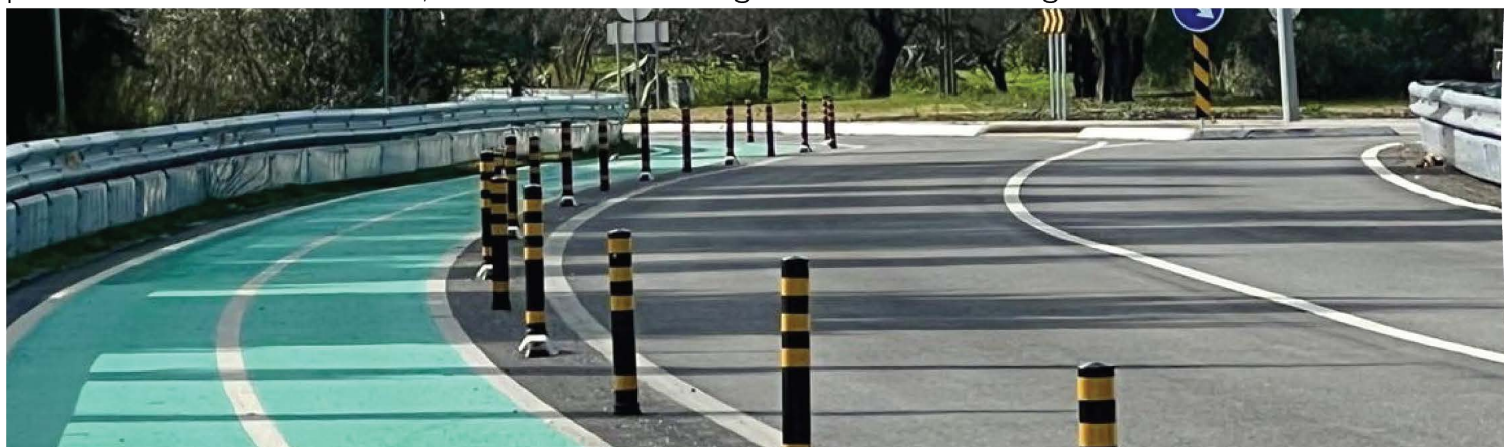
Bidirectional protected cycleway on an urban arterial - A Continuous, unambiguous edge at vehicle mirror height.
